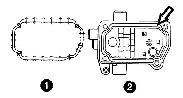
In view of the fact the the new gasket necessitates a widening of the groove in the housing cover (item 2), the gasket used to date will continue to remain a valid service part.
